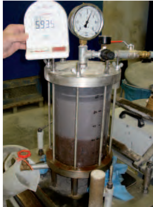
Laboratory mortar drain test with soil sample
